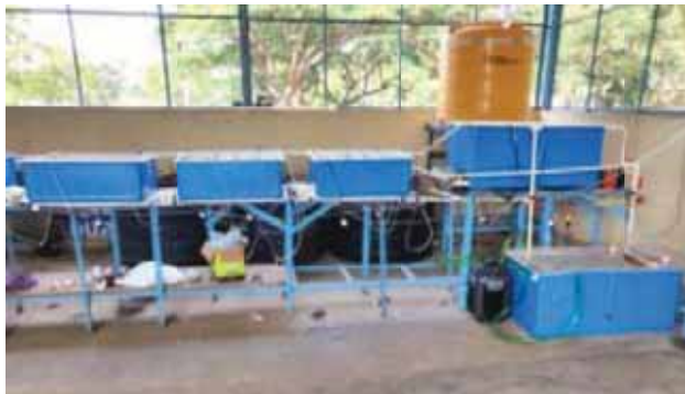
Fig.13.11 Re-circulatory egg hatching system
