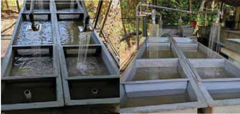
Fig.10.5 FRP tank with incubation tray
